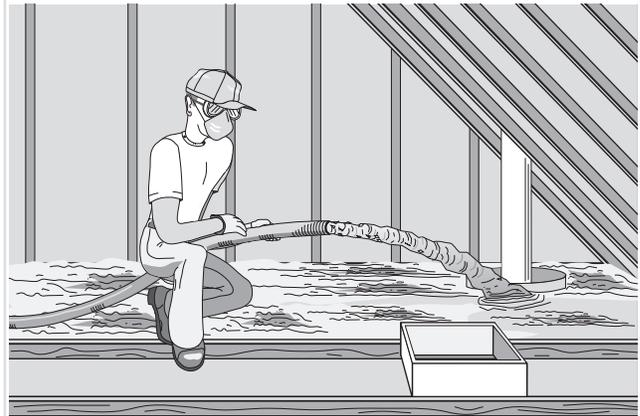
*Either loose-fill fiberglass or loose-fill cellulose insulation are good choices for attic insulation because they form a seamless blanket. Insulation dams are installed to maintain clearance around the attic hatch and chimney.*
